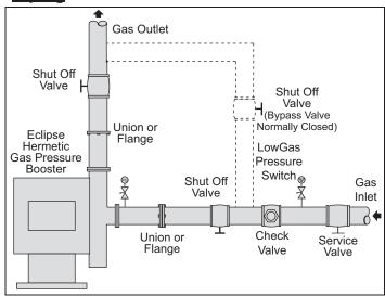
Figure 1. Typical Piping Arrangement
