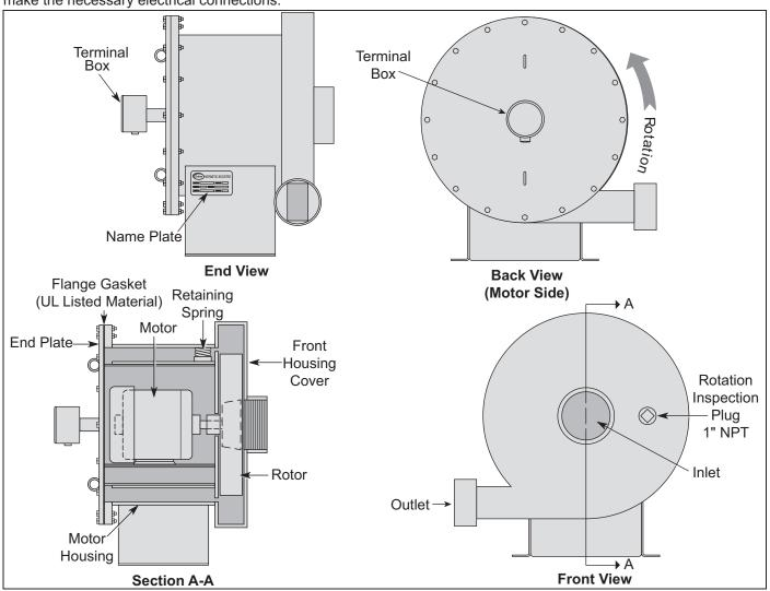
Figure 2. Parts Identification & Location - HB Series
